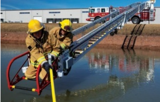
Below grade operation (-10 degrees)
